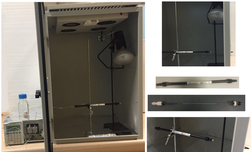
Fig. 1. A photograph of the microfluidic packed bed reactor (MPPBR) system used for continuous photodecolorization of RB5 solution.
