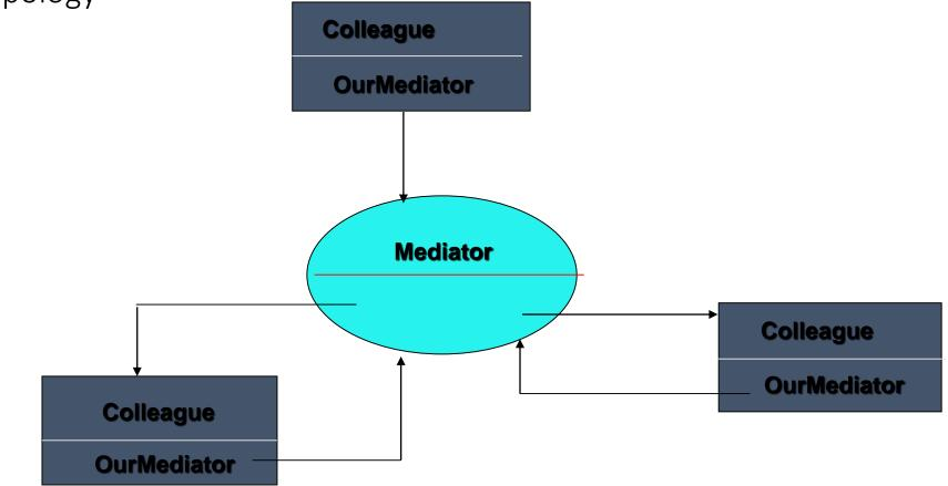
Provides a common connection point, centralized (subclassable) behavior and behavior mgmt, all with a common interface
