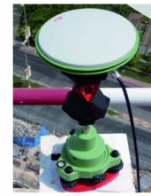
b. GNSS antenna coupled with 360° prism reflector.
