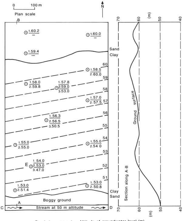
Borehole 1.57.8 1. = Altitude of groundwater level (m) 2.59.0 2. = Altitude of top of sand layer (m)
