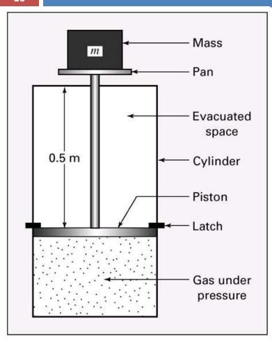
Piston-cylinder arrangement contains nitrogen gas trapped below the piston at 7 bar. Piston is held in place by latches. Space above the piston is evacuated. A pan is attached to the piston rod and a mass m of 45 kg is fastened to the pan. Piston, rod and pan together are 23 kg. Latches holding the piston are released, allowing the piston to rise rapidly 0.5 m until it strikes the top of the cylinder. What are the energy changes?
