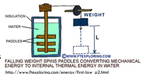
Temperature of water rises due to stirring, i.e. friction between the water and the paddles.
