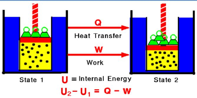
Any thermodynamic system in an equilibrium state possesses a state variable called the internal energy (U). Between any two equilibrium states, the change in internal energy is equal to the difference of the heat transfer into the system and work done by the system.
