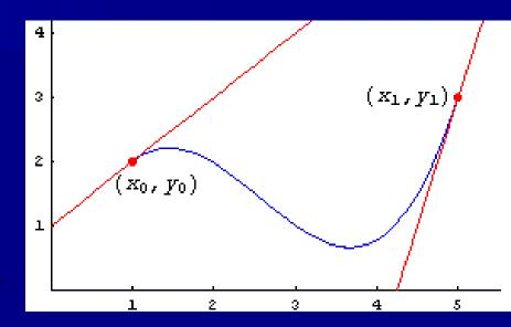
If f[x] is continuous on [x<sub>0</sub>,x<sub>1</sub>], there exists a unique cubic polynomial p[x]=ax<sup>3</sup>+bx<sup>2</sup>+cx+d such that p[x<sub>0</sub>]=f[x<sub>0</sub>] p[x<sub>1</sub>]=f[x<sub>1</sub>] p'[x<sub>0</sub>]=f'[x<sub>0</sub>] p'[x<sub>1</sub>]=f'[x<sub>1</sub>]
