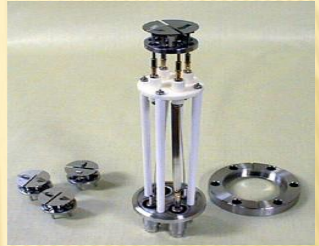
Figure 3 - Basic electron gun
