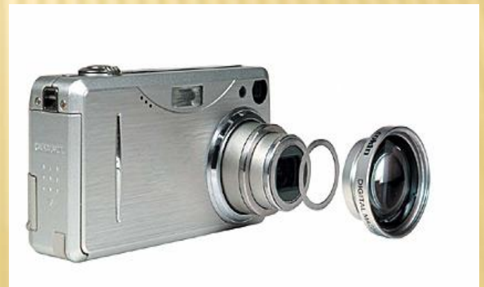
Figure 4 - Magnetic lens on camera
