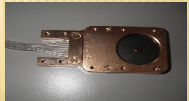
Figure 6 - MCP (Microchannel Plate) Detectors For SEM and CD-SEM
