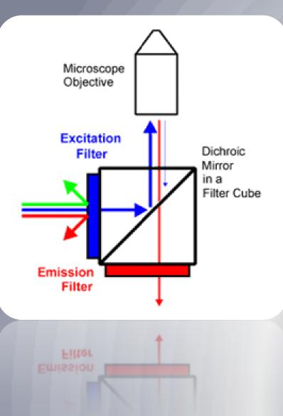
✓ The dichroic mirror is mounted on an optical block commonly referred to as a filter cube.
