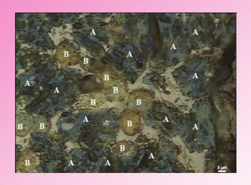
View of branded clinker with nitric acid (50 times enlarged A:Alit cristals, B:Belit cristals)
