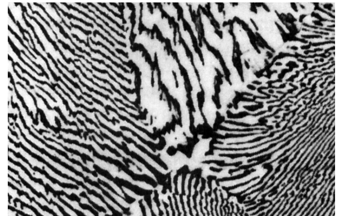
Microstructure of Pb-Sn eutectic lamellae
