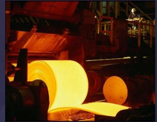
Aluminum is hot rolled into a coil of desired thickness.*
