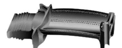
A blade with internal cooling as applied in the highpressure turbine
