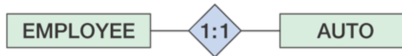
Figure 2.7 Three Types of Binary Relationships (a) 1:1 Binary Relationship; (b) 1:N Binary Relationship and (c) N:M Binary Relationship
