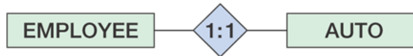
Figure 2.7 Three Types of Binary Relationships (a) 1:1 Binary Relationship; (b) 1:N Binary Relationship and (c) N:M Binary Relationship
