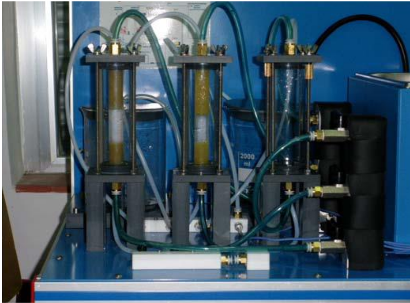
Figure 14. Installed reactors (2 catalytic reactors with different grain size and 1 enzymatic reactor).
