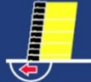
c) bearing capacity (excessive settlement)
