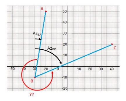
Angle to the right at point B =  $Az_{BC}-Az_{BA}+360^{\circ}$   $\alpha = atan [(E_A-E_B)/(N_A-N_B)] = atan [(-20-(-30))/(50-(-10))] = atan (10/60) = 9.46^{\circ}$ If both  $\Delta E$  and  $\Delta N$  are positive, then  $Az_{BA} = 9.46^{\circ}$   $\alpha = atan [(E_C-E_B)/(N_C-N_B)] = atan [(40-(-30))/(20-(-10))] = atan (70/30) = 66.80^{\circ}$ If both  $\Delta E$  and  $\Delta N$  are positive, then  $Az_{BC} = 66.80^{\circ}$
