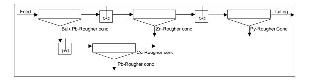
Bulk Flotation: All valuable minerals (Pb + Zn + Cu + Ag + Au ..) may be floated together into the same mixed bulk concentrate. This can be necessary due to the complex nature of the ore or for economic reasons.
