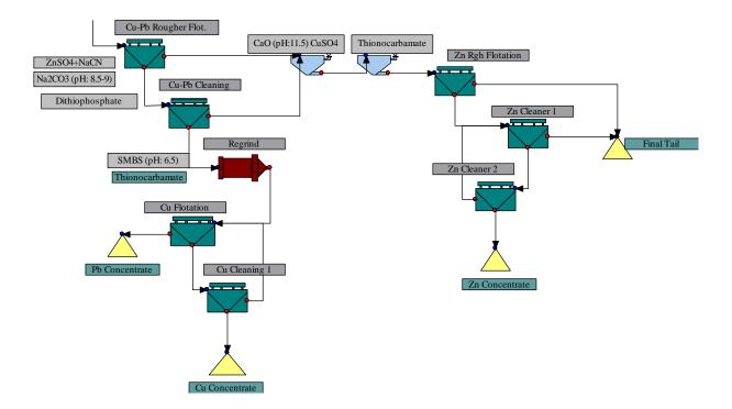
An example of Differential Flotation of Copper-Zinc-Lead Sulphide Flotation Circuits
