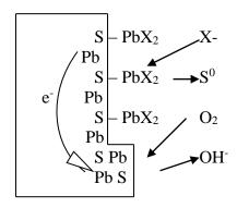
In this model the role of the oxygen is to oxidise lattice sulphide ion to sulphur.
