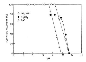
The pzc for pyrite is at pH = 6.9. Above pH 6.9 the surface of the pyrite is negatively charged and Ca<sup>2+</sup> adsorbs readily by electrostatic attraction and this hinders the oxidation reaction on the pyrite surface.
