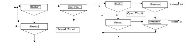
There are many circuits now arranged in an open circuit arrangement as shown above. This has two advantages.
