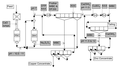
This example of a mixed sulphide circuit shows a typical arrangement of reagent addition points for the flotation separation.
