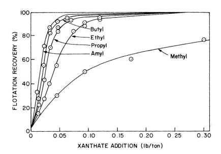
For example, with the same concentration of  $Pb_2^+$ , a smaller concentration of amyl xanthate (C5) is required to form a precipitate of lead amyl xanthate than is required to form lead ethyl xanthate with ethyl xanthate.
