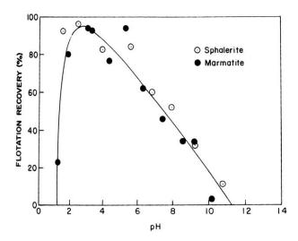
At higher concentrations of longer chain xanthates sphalerite responds quite readily to flotation
