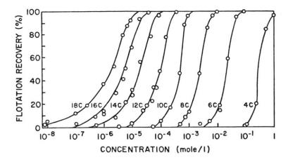
Flotation of quartz in aminium acetate solutions at neutral pH
