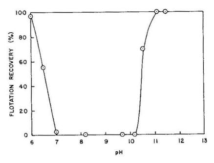
Flotation of calcite with 5x10<sup>-4</sup> oleate and 5x10<sup>-4</sup> sodium silicate
