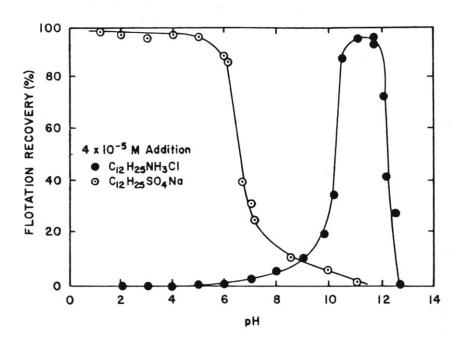
Flotation recovery of corundum (Al<sub>2</sub>O<sub>3</sub>) with 4x10<sup>-5</sup>M additions of collector
