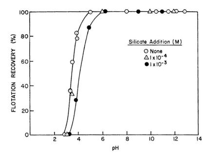
Flotation of apatite with 1x10<sup>-4</sup>M oleate with and without silicate addition
