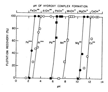
Minimum pH for flotation of quartz with 1x10<sup>-4</sup>M sulphonate and 1x10<sup>-4</sup>M metal ion
