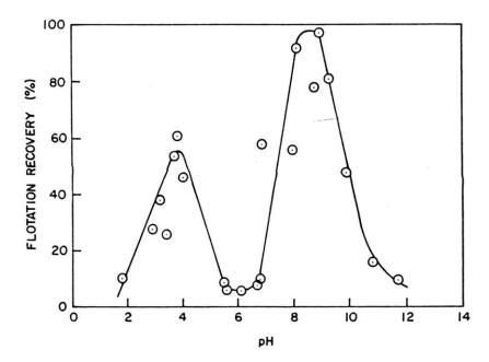
Flotation of pyrolusite (MnO<sub>2</sub>) with 1x10<sup>-4</sup>M acetate
