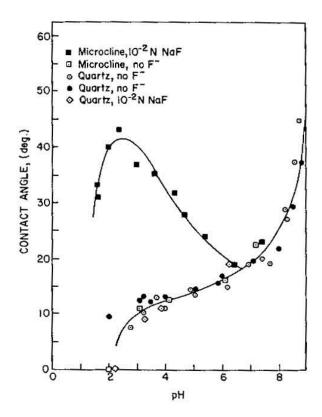
Contact angle of feldspar (microcline) and quartz showing effect of fluoride
