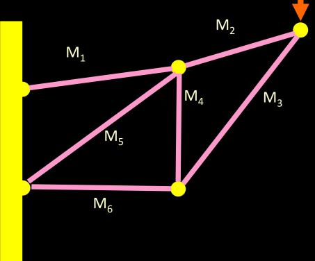
Pins transfer force between beams. If the truss is in equilibrium, all forces acting on a pin must sum to zero.
