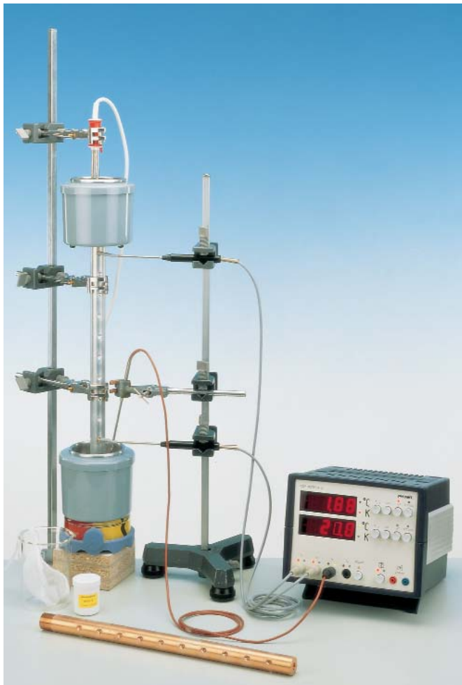
Fig. 1a: Experimental set-up for thermal conductivity.
